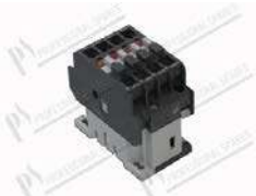
Schütz AF12-30-10-11 5,5kW 3P; 230V 50/60Hz 400V 3 cont. NO + 1 aux NO
