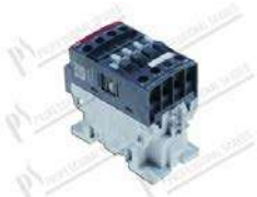
Schütz A9-30-10 4kW 3P; 24VAC 50/60Hz; 400V 3 cont. NO + 1 aux NO; dim. 75x43x72 mm
