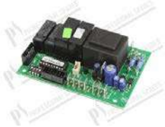
Motherboard 230V 50/60Hz BHC / C / FC / GF / LB / LC / LF
