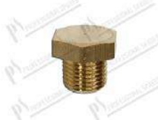
Plug G1/8" - brass H=12 mm; CH13
