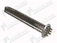
Boiler heating element 5000W 230V L=253 mm; flange Øest. 64 mm Øint. 47,5 mm; bulbe housing, fastons 6,3x0,8 mm
