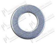
Flat washer M8 Ø 8,5x15,7x1,4 mm INOX
