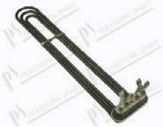
Tank heating element 3000W 230/400V L=380 mm; flange 80x25 mm
