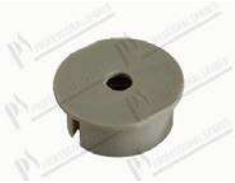
Plug for overflow pipe Ø 60 mm H=25 mm hole Ø 12,3 mm
