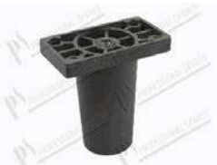
Foot support plastic H=116,5 mm flange 109x60 mm; thread M10
