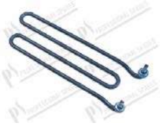
Tank heating element 2000W 230V dim.318x85xh26mm; connection M12
