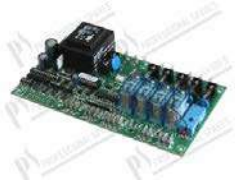
Motherboard 180x100 mm FC5 / GF90 / LF320LA / LF400A
