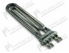
Heizkörper boiler 5600W 230V dim. 270x65 mm; flansch 81x28 mm
