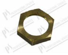
Hexagonal nut 1 1/4 - brass Ø 33,6 mm; H=12 mm; CH46
