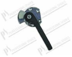
Oven door handle - right side handle L=170 mm - flange 80x69 mm - 4 holes Ø 6,5 mm
