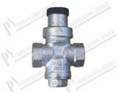
Water pressure reducer 1/2"FF setting range 1.0 to 4.0 bar; Maximum inlet pressure 10 bar
