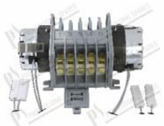
Timer chambers 5 120 - 6 sec. 230V 50/60Hz; cable L=280 mm faston F 6,3 mm
