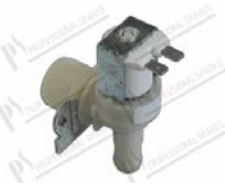
Solenoid valve 90° - 1 way - 220/240V 50/60Hz - Ø 14 mm with fastons; inlet Ø 3/4" with filter and inlet reducer 20 lt/min; Tmax 90°C
