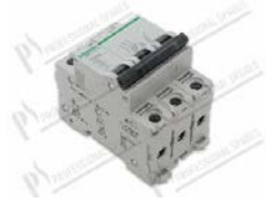
Automatic circuit breaker 3P 20A 400V dim. 75x53x81 mm
