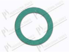
Joint plat Ø 21,5x30x2 mm - Fibre
