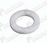
Joint plat Ø 15,2x24,2x2,8 mm
