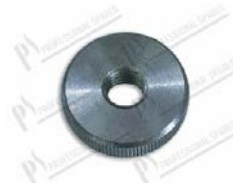
Knurled nut M5x0,75 Ø 19,5 mm H=4 mm
