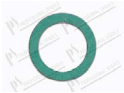
Flat gasket Ø 14,5x22x1,7 mm - Fiber
