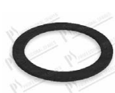
Flat gasket Ø 47,5x60x1,9 mm - EPDM
