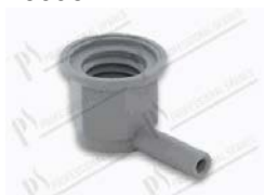
Air break connection 90° M13x2 rubber holder Ø 5,6 mm
