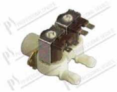
Solenoid valve 180° - 2 way - 200-240V 50/60Hz - Ø 10,5 mm with fastons; inlet Ø 3/4" with filter and reducer 14 lt/min; Tmax 90°C
