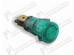
Green pilot lamp Ø 13 mm 230V self-locking lens Ø 15 mm; L=33 mm; faston 6,3x0,8 mm; Tmax 120°C
