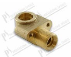
Level viewer adapter 90° 3/8" - brass hole Ø 13,5 mm
