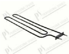
Heating element 1000W 230V dim. 512x120 mm; flange 77x21 mm; faston 6,3 mm
