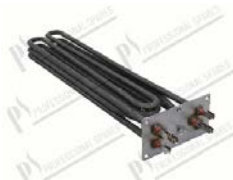
Boiler heating element 9000W 230V dim. 385x80 mm; flange 105x55 mm; faston 6,3 mm
