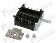
Commutator 0-1 positions 16A 250V; Tmax 150°C; D shaft Ø 6X4,6 mm
