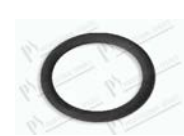
O-ring 3,53x24,99 mm NBR
