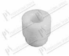
Lower bushing Ø 25x51x51 mm thread 1" 1/4
