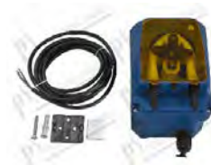
Detergent peristaltic pump w/speed adj. (external use) mod. PR-7; flow rate from 1÷7 lt/h press. 0,1 bar; 230V 50Hz; protection IP65; hose in Santoprene with rubber holder Ø 6,2x10,2 mm for hose clamp; cable L=2750 mm; installation kit included
