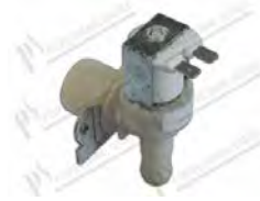
Solenoid valve 90° - 1 way - 220/240V 50/60Hz - Ø 14 mm with fastons; inlet Ø 3/4" with filter and inlet reducer 20 lt/min; Tmax 90°C
