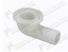
Rubber holder 90° 3/4" F - outlet Ø 21 mm
