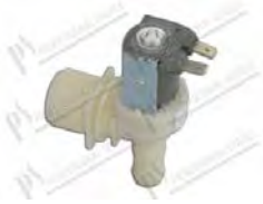
Solenoid valve 90° - 1 way - 24Vac 50/60Hz - Ø 14 mm with fastons; inlet Ø 3/4" with filter; Tmax 90°C
