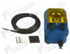
Detergent peristaltic pump w/speed adj. (external use) mod. PR-7; flow rate from 1÷7 lt/h press. 0,1 bar; 230V 50Hz; protection IP65; hose in Santoprene with rubber holder Ø 5x8 mm; cable L=2750 mm; installation kit included
