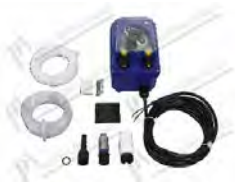
Rinse aid peristaltic pump w/speed adj. (external use) mod. PR-1; flow rate adj. from 0,15÷1 lt/h press. 3 bar; 230V 50Hz; protection IP65; cable L=1200 mm; Hose in sekobrill; installation kit included
