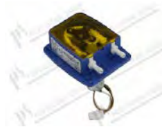
Detergent peristaltic pump fixed capacity mod. PP; fixed flow rate 7 L/h; 0,1 bar; 24V 3,5W; hose in Santoprene ; Cable L=205mm
