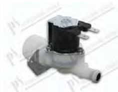
Solenoid valve 180° - 1 way - 24Vdc 50Hz - Ø 10,5 mm with fastons; inlet Ø 3/4" with filter; and reducer 10 lt/min; outlet 2,5 lt/min; Tmax 90°C - (RPE)
