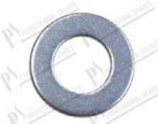
Flat washer M8 Ø 8,5x15,7x1,4 mm INOX
