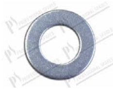
Flat washer M8 Ø 8,5x15,7x1,4 mm INOX
